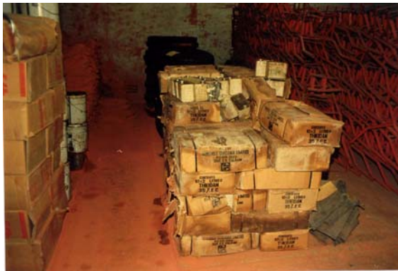
Inappropriate containers may be damaged in store leading to leakage, contaminating warehouse environment and items stored together with the pesticides.
